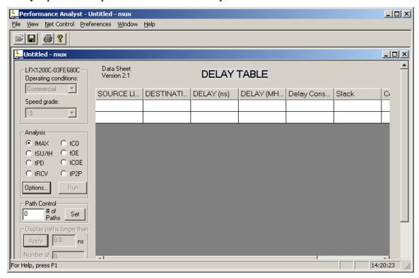
The Performance Analyst performs eight distinct analyses: fMAX, tSU/tH, tPD, tRCV, tCO, tOE, tCOE, and tP2P. The first type, fMAX, is an internal register-to-register delay analysis. fMAX measures the maximum clock operating frequency, limited by worst-case register-to-register delay. The remaining seven types are
