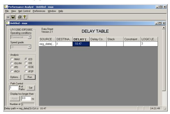
4. Click the highlighted cell (**10.47**) in the spreadsheet window to open the Expanded Path dialog box.
