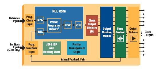
Figure 2 - Block diagram of ispClocK5620
