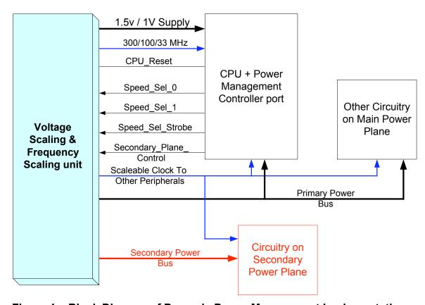
Figure 1 – Block Diagram of Dynamic Power Management Implementation
