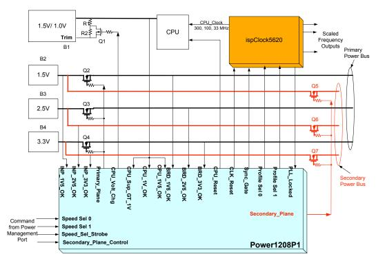
Figure 3 - Voltage Scaling and Frequency Scaling Unit
