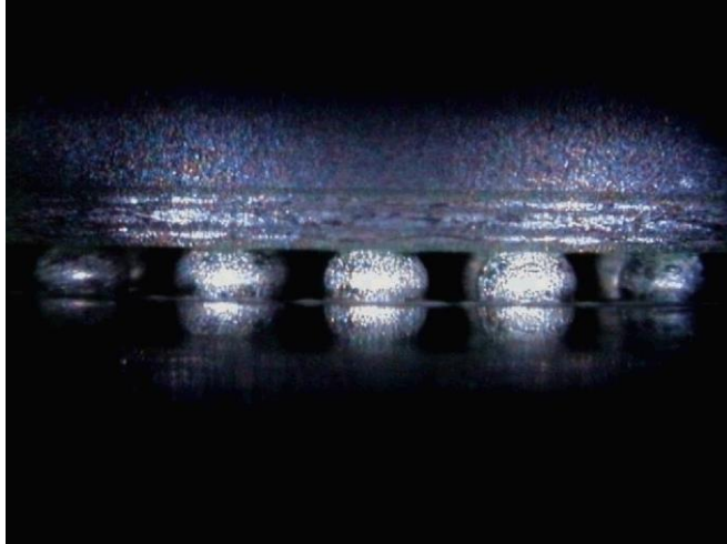
Figure 8.5. Edge View Camera Inspection
