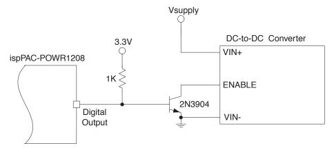
In this circuit, the maximum sink current is determined by transistor's base drive current (~2.5mA) multiplied by its gain, and can easily be in the tens or even hundreds of mA. The maximum allowable off-state voltage also increases to the external transistor's collector breakdown voltage, in this case approximately 40V. Note that the external transistor is turned ON (shorting the converter ENABLE line to ground) when the ispPAC-POWR1208's output is HIGH.
