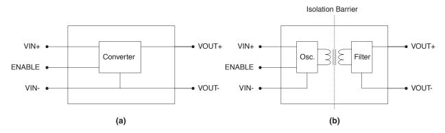
In the case of non-isolated converters, the ENABLE line is electrically referenced to both VIN- and VOUT-, so as long as the control circuitry is 'ground' referenced to either of these pins, no special measures need to be taken beyond assuring compatible voltage and current levels.
