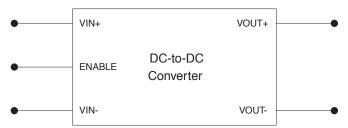
While the ENABLE inputs of some converter modules accept standard (5V or 3.3V) logic levels, many other electrical interfaces are common as well. The purpose of this applications note is to describe how to interface the logic outputs of Lattice Semiconductor's ispPAC-POWR1208 to some of these non-standard interfaces.
