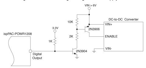
In this circuit, the collector of the NPN transistor now stands-off the VIN+ voltage instead of the ispPAC-POWR1208's output, offering compatibility with higher VIN+ voltages, depending on the choice of transistors. The addition of the extra transistor also has the effect of inverting the ispPAC-POWR1208's digital output, so that the PNP transistor is now turned ON when the digital output is HIGH. Note that a similar solution using opto-couplers will be discussed later in this application note.
