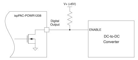
For converters with non-standard inputs requiring either an open state or short-to-ground, the circuit of Figure 3 can also be used if one removes the pull-up resistor. In this case, the converter must have the following characteristics:
