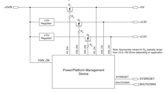
If an over-voltage condition is seen, the specified action will be to turn everything off fast and HALT. This can be accomplished with minimal changes to the sequence by specifying an exception. Exceptions are listed in Logi-Builder in the exception table (Figure 8), which is displayed immediately beneath the sequence table. Each exception occupies one row in the exception table.
