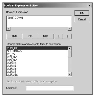
This dialog box allows the user to specify a Boolean expression for which the sequence must wait to become true before it continues. An expression may be constructed either by typing it in free-form in the top editing field, or may be built by selecting listed variables (by double-clicking on the desired variable) and operators (AND, OR, NOT, '(', ')'). This dialog also provides an editable field for adding comments to the LogiBuilder sequence.
