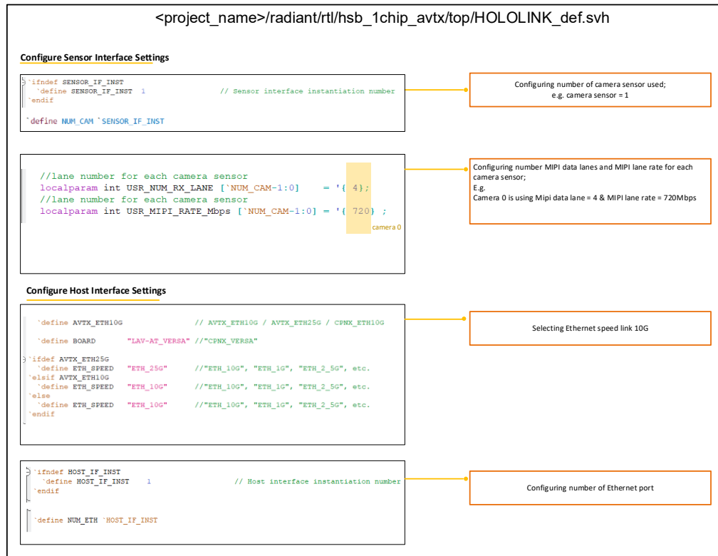
Figure 4.10. Required HDL Parameter and DEFINE Switch Configuration
