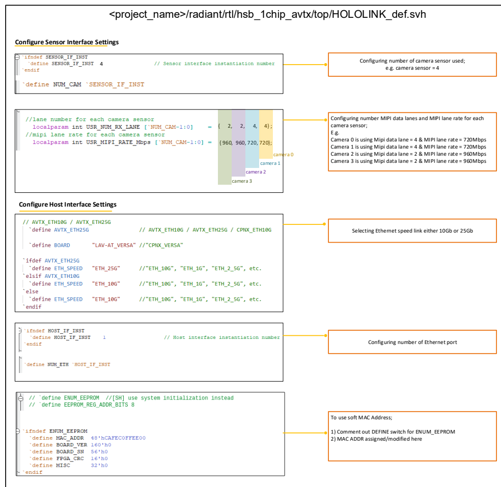
Figure 4.5. Define Switch Setting in HOLOLINK_def.svh File
