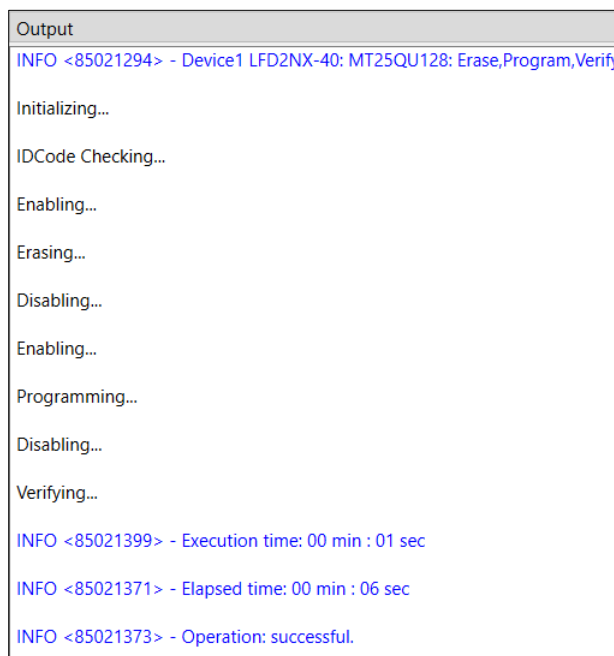
Figure 6.18. Radiant Programmer Console Output after Programming the SPI Flash
