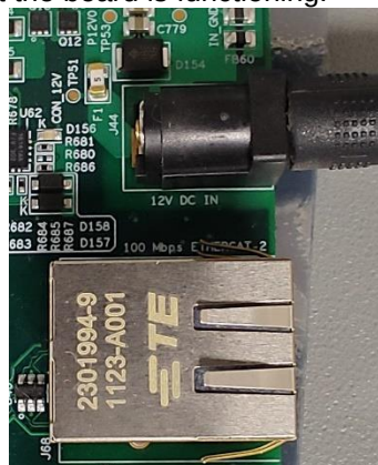
Figure 3 12 V DC Power Supply
