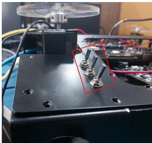
Figure 7.45. Three Resistor Switches Tilted Towards the Resistors
