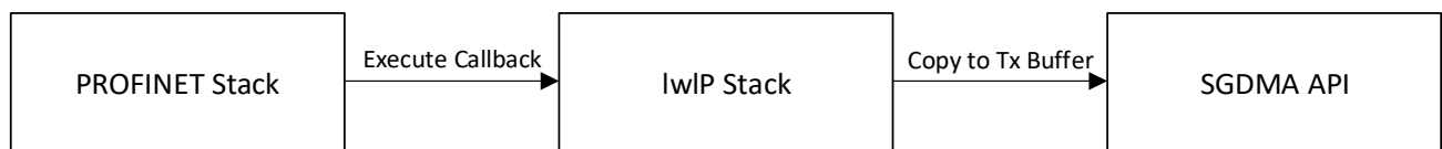
Figure 4.2. SGDMA Driver API Transmit
