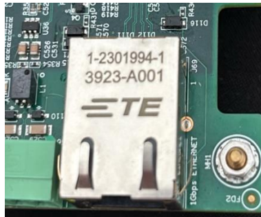
Figure 4.4. ADIN1300 Ports Located on the ADI MCB
