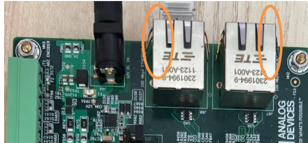
Figure 4.3. ADIN1200 Ports Located on the ADI MCB
