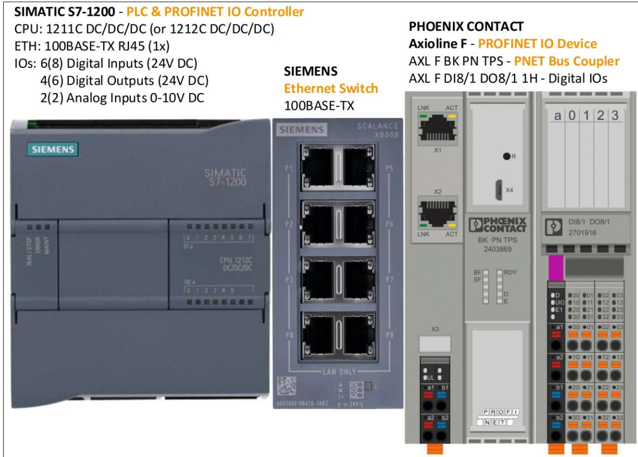
Figure 7.2. PROFINET Demo Hardware Setup
