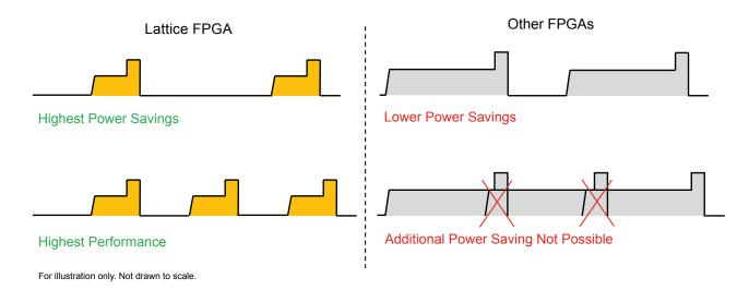
Comparing the total power (area under the curve), it is evident that Lattice Nexus 2 devices can power duty-cycle while maintaining a high level of performance in edge monitoring applications.
