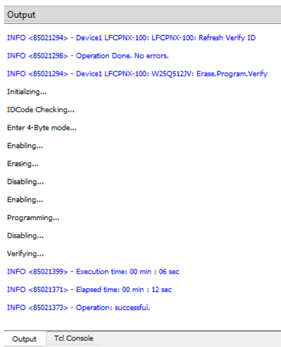
Figure 7.37. Radiant Programmer Console Output after Programming
