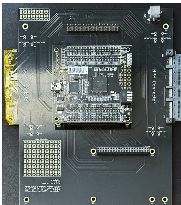
Figure 5.4. Assembled LTPI Demonstration Board
