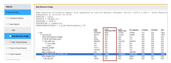
If distributed RAM is used in the design, there are four separate workarounds that can be used to avoid this issue.
