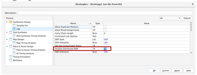
Note: If the design includes Lattice or 3<sup>rd</sup> party IP that uses Distributed RAM that has data widths that are not a multiple of 4, please contact <u>Lattice Technical Support</u>.
