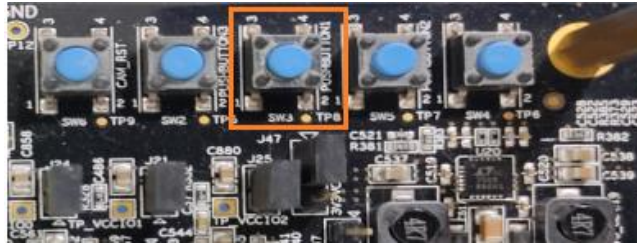
Figure B.23. Button SW3 of Certus NX Versa Board
