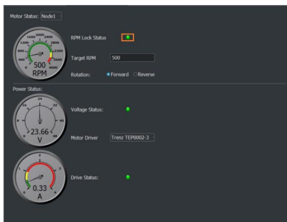
Figure 7.25. User Interface Application Motor Status: RPM Lock Status When Target RPM is Achieved
