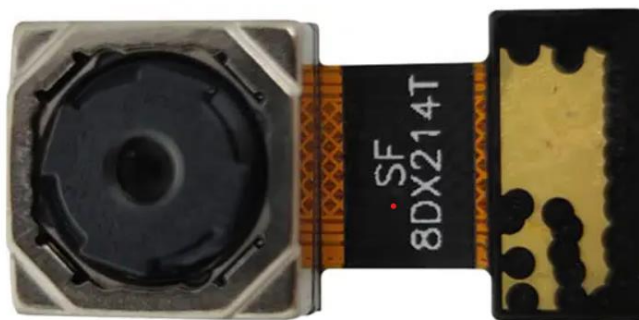
Figure 3.1. Sony IMX214 Camera
