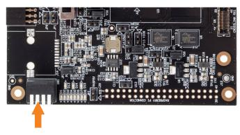
Figure 6.10. Switch to Send Broadcast Command Using the MachXO5-NX Initiator
