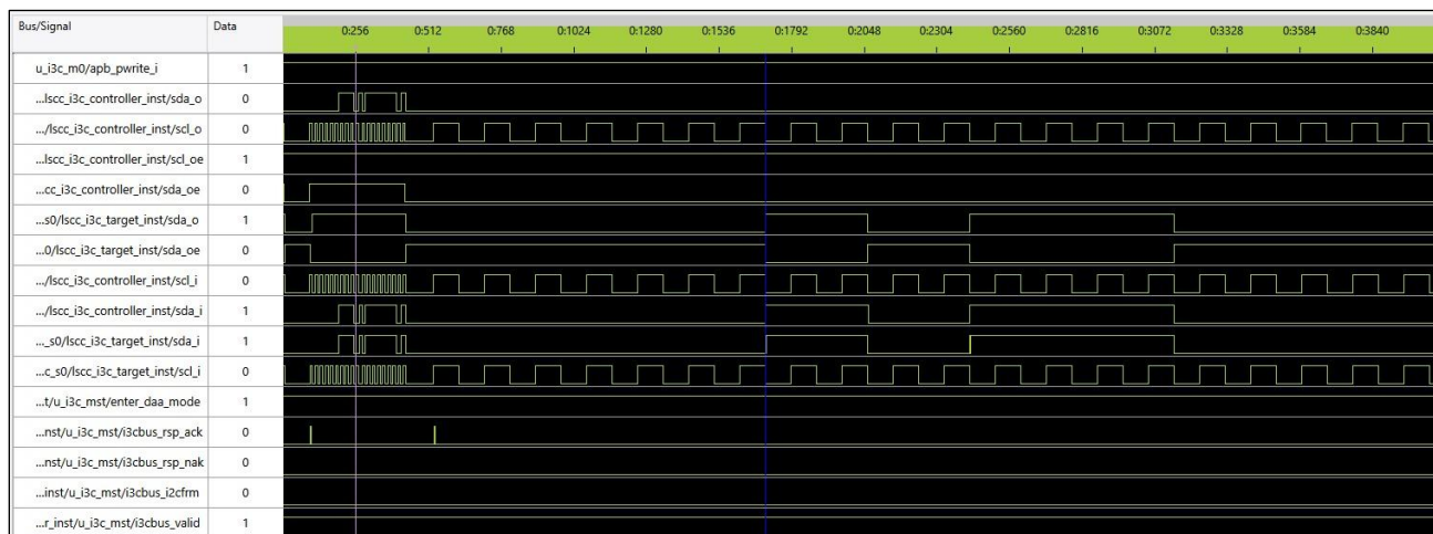
Figure 6.9. Sample ENTDA sequence sent by I3C Controller
