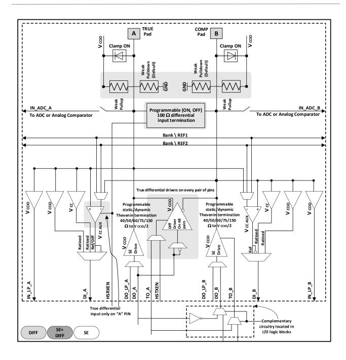
Figure 8.1. High-Performance sysI/O Buffer Pair for Bottom Side
