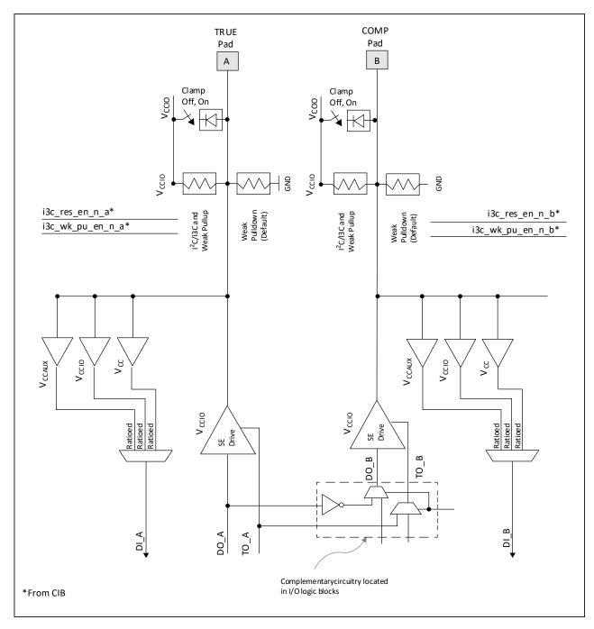
Figure 8.2. Wide Range sysl/O Buffer for Top, Left / Right Side
