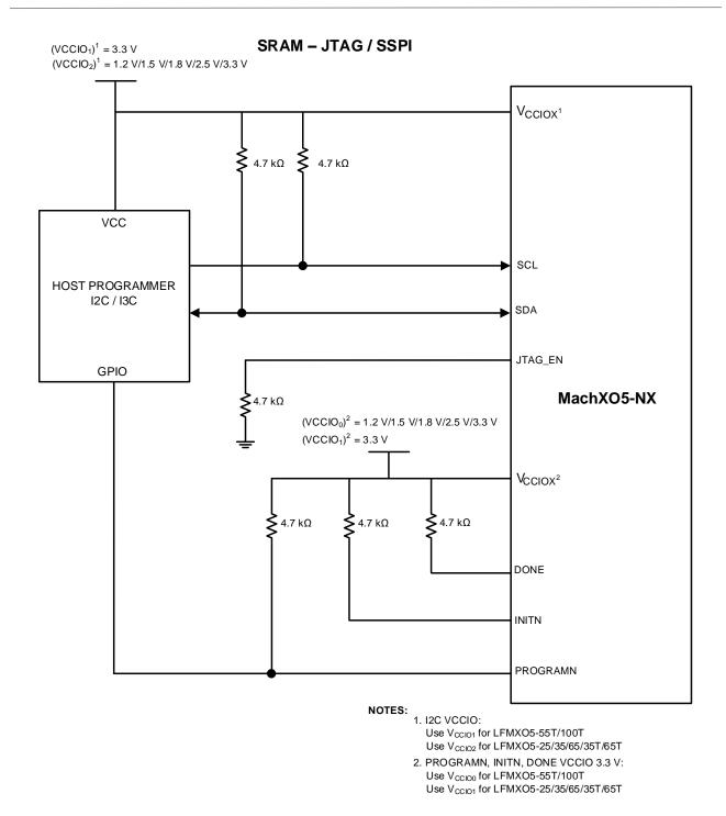
Figure 6.2. Typical Connections for Programming SRAM / FLASH via I2C / I3C
