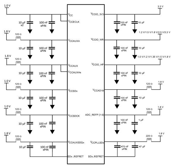
Figure 3.1. Recommended Power Filter
