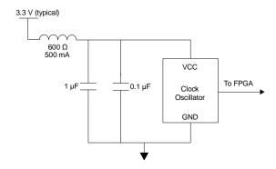
Figure 9.1. Clock Oscillator Bypassing
