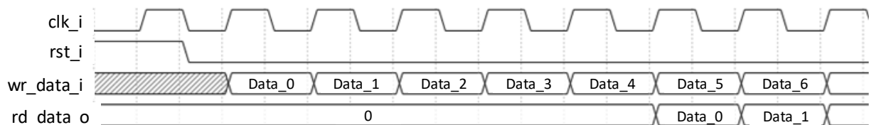
Figure 2.20. Shift Register Without Output Register (LUT Memory, iCE40UP Devices)
