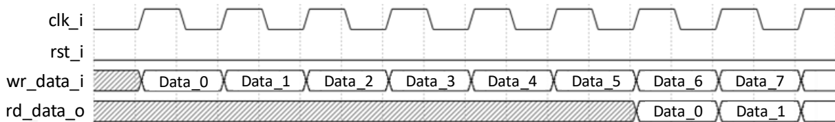
Figure 2.17. Shift Register With Output Register
