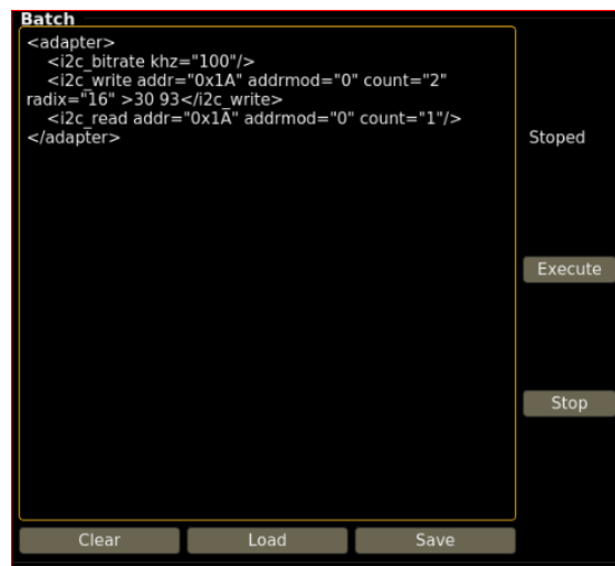
Figure 6.25. I2C Batch Mode Read/Write
