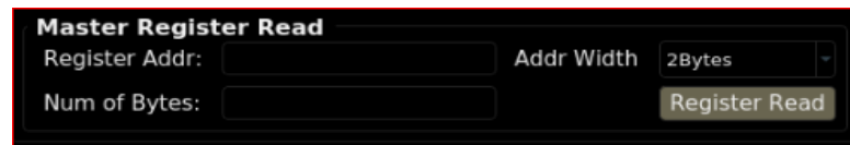
Figure 6.20. I2C Master Register Read
