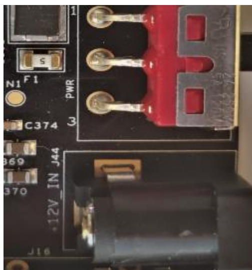
Figure 1.3. 12 V DC Power Supply
