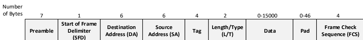
Figure 2.3. Tagged Ethernet Frame Format
