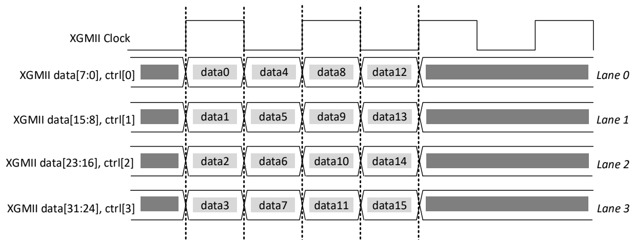
Figure 2.3. XGMII Timing Diagram
