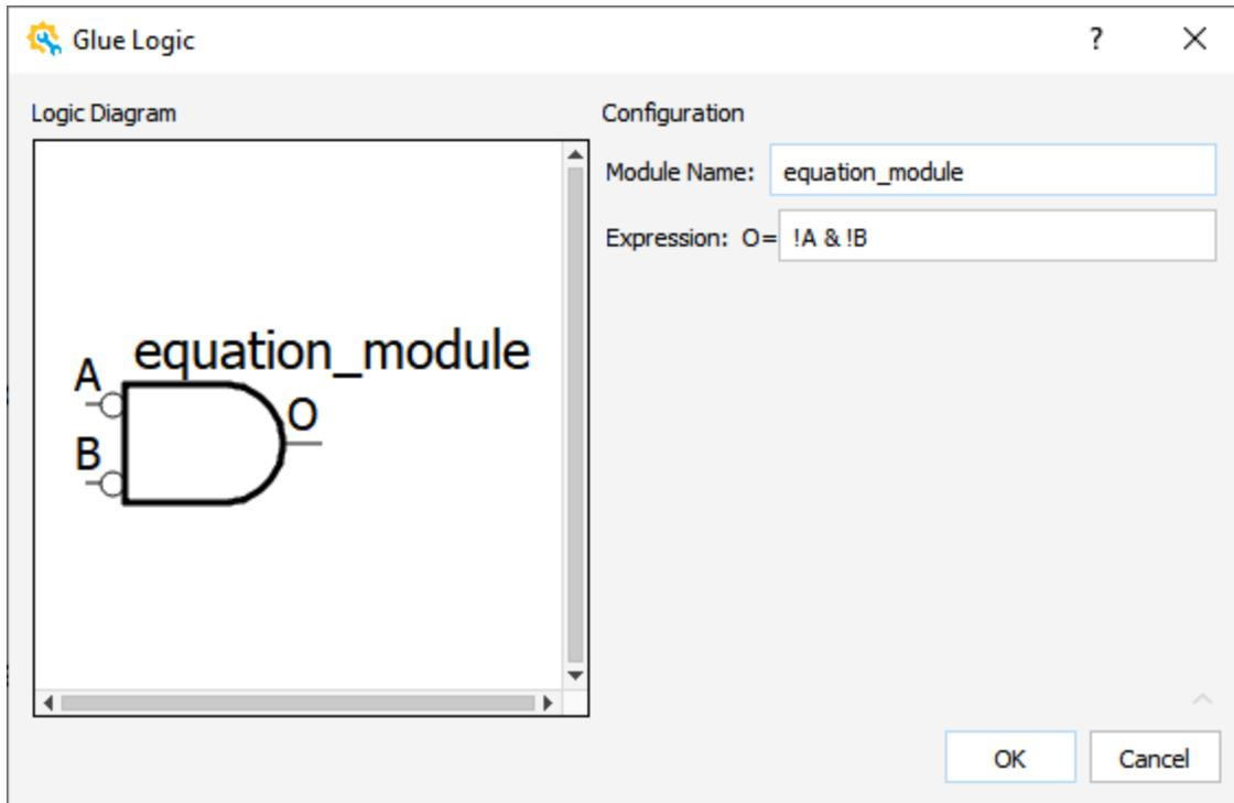
Figure 2.23. Glue Logic Wizard for Equation Module
