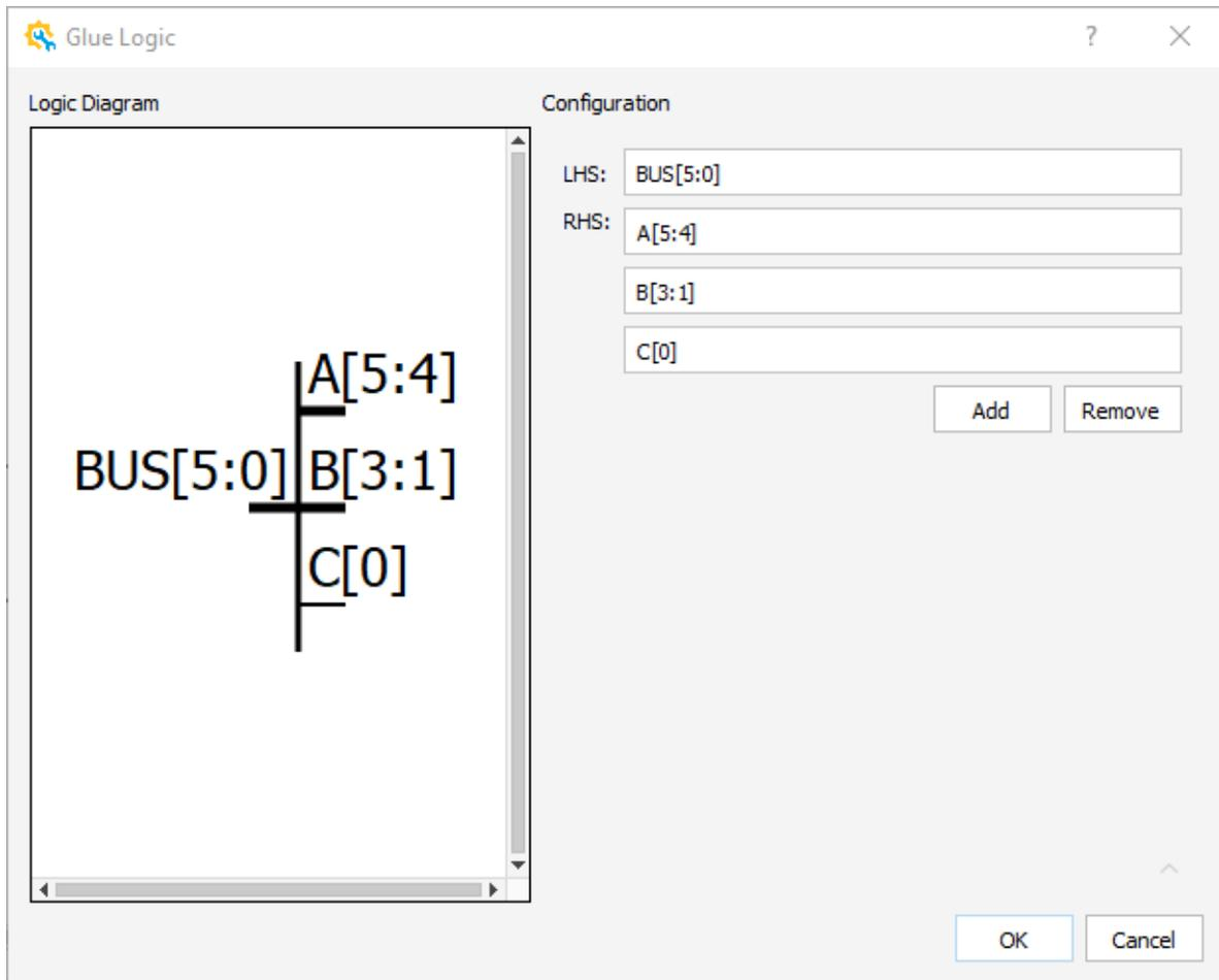
Figure 2.29. Glue Logic Wizard for Split Module
