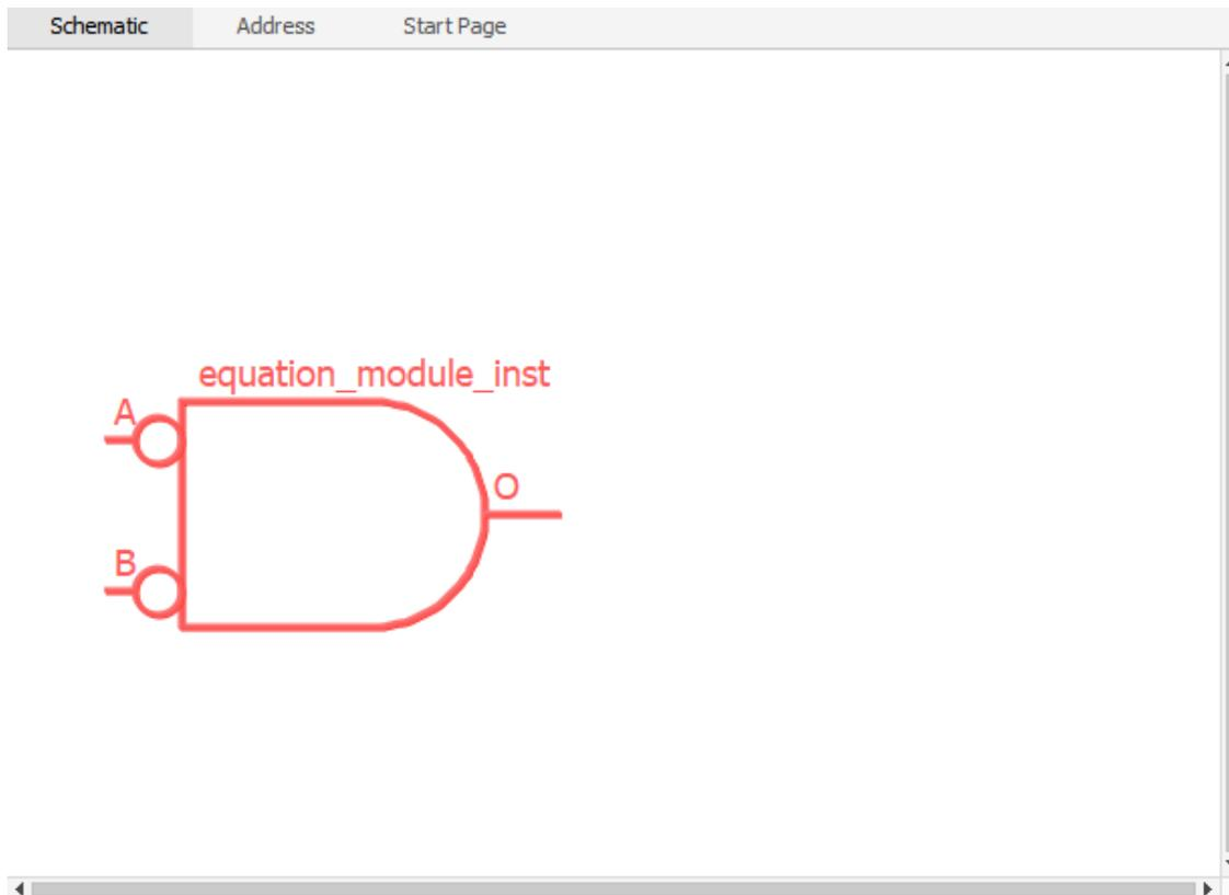
**Figure 2.24. Schematic View Shows an Equation Module**
