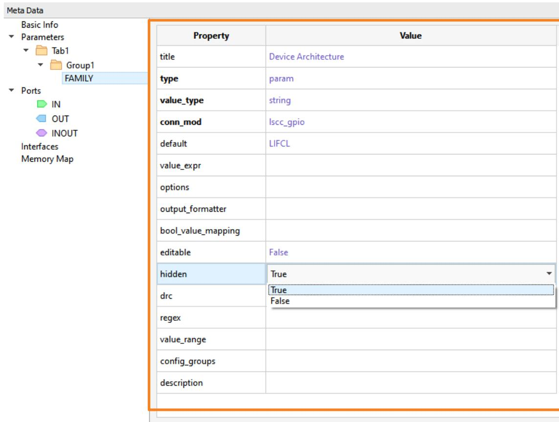
Figure 3.14. Configure a Parameter
