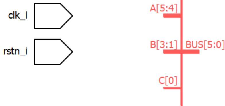
**Figure 2.22. Schematic View Shows a Concat Module**
