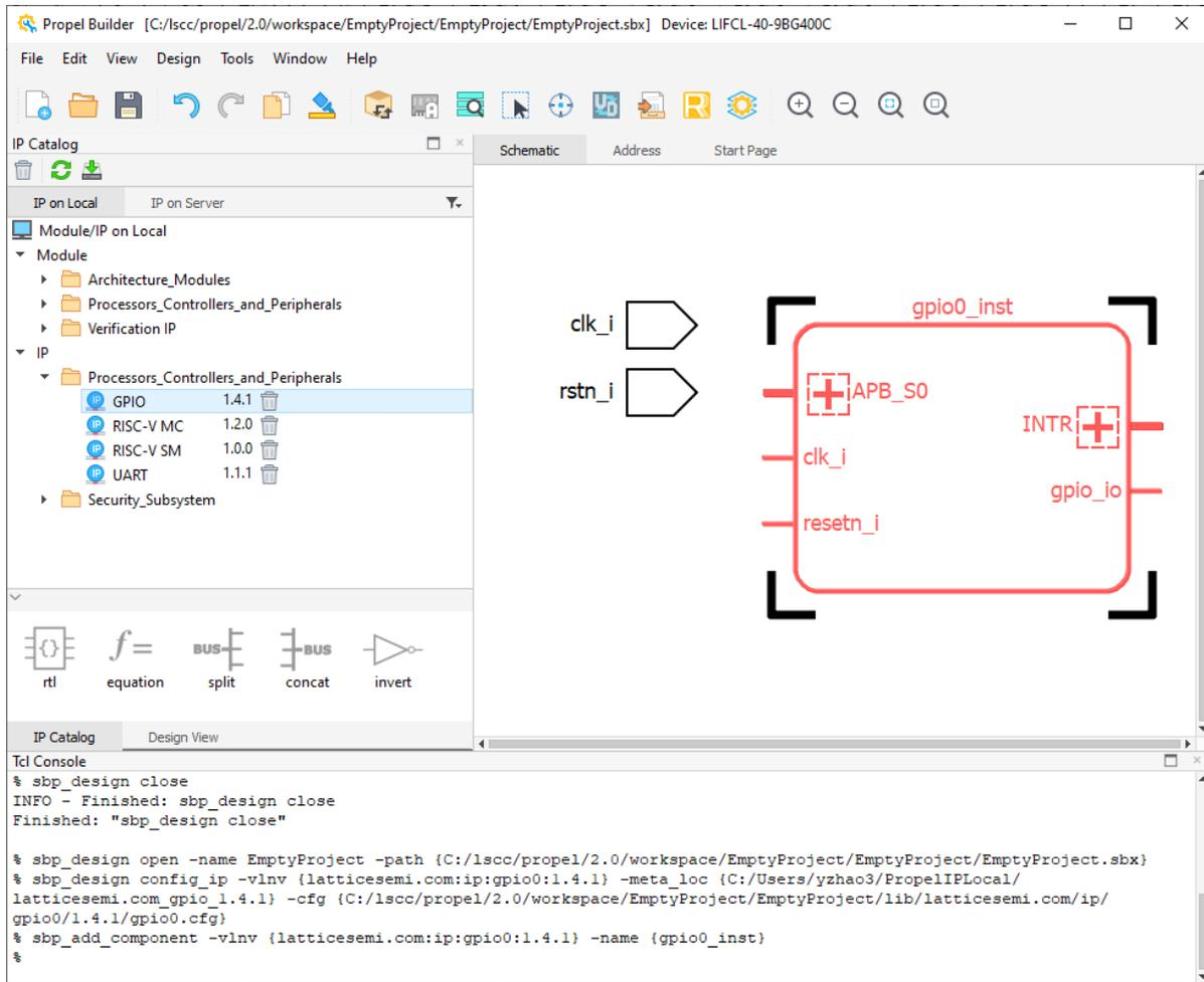
Figure 2.19. Propel Builder Schematic View Shows the Module Instance
