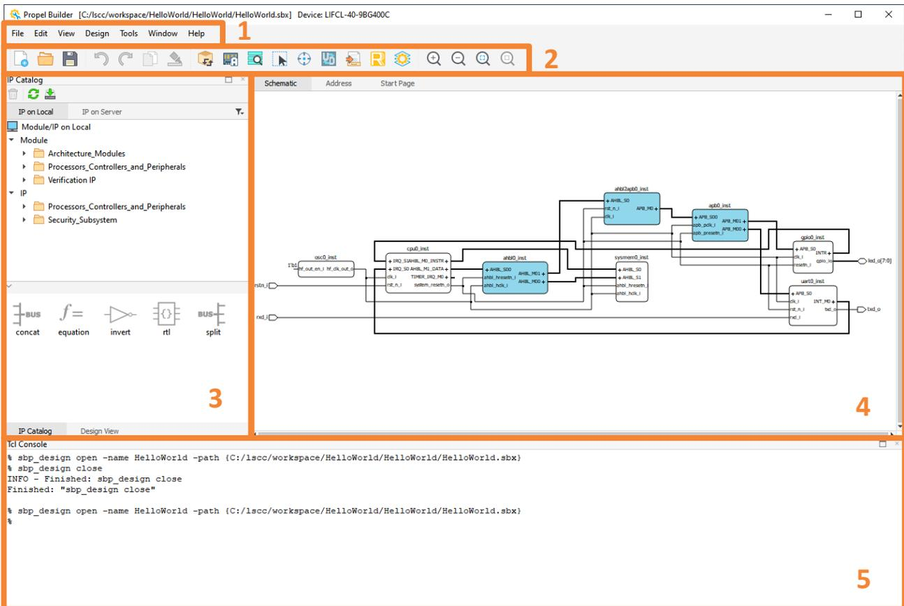
Figure 2.1. Propel Builder Workbench Window
