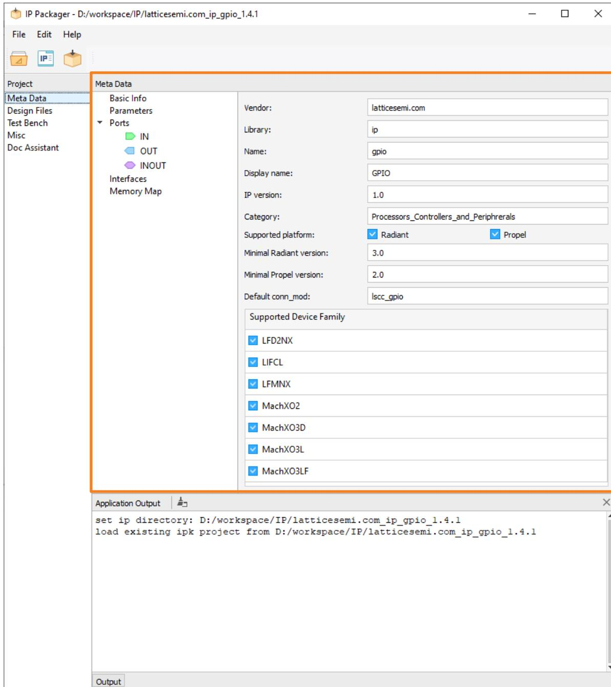
Figure 3.6. IP Packager with Meta Data Details
