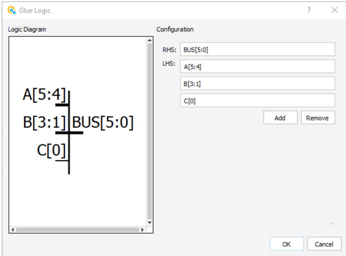
**Figure 2.21. Glue Logic for Concat Module**
