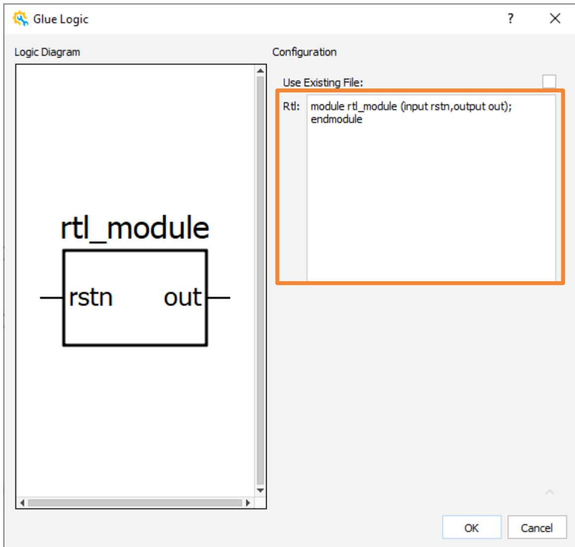
**Figure 2.26. Glue Logic Wizard for Rtl Module**
