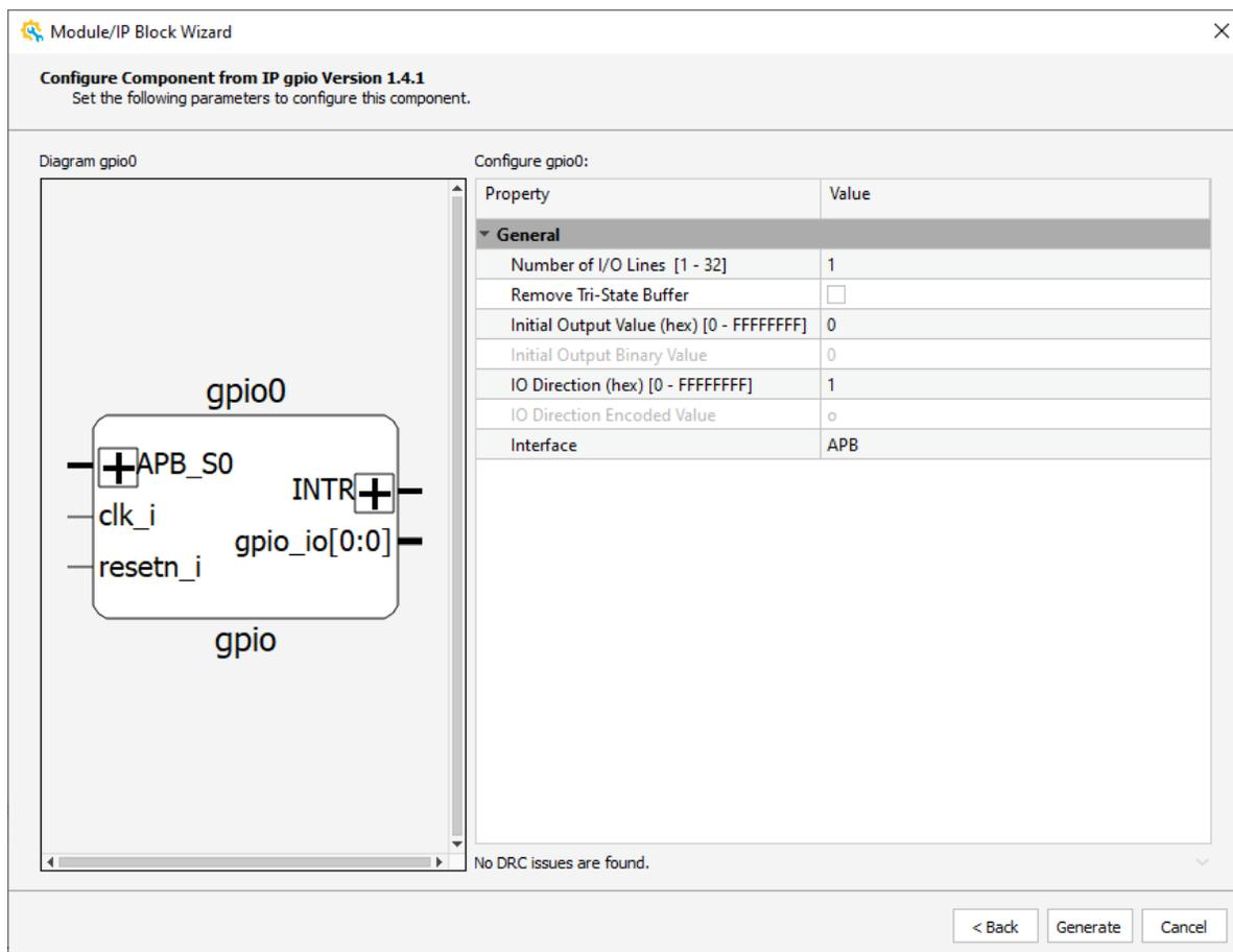
Figure 2.16. Module/IP Block Wizard - Configure Component from IP Gpio Version 1.4.1
