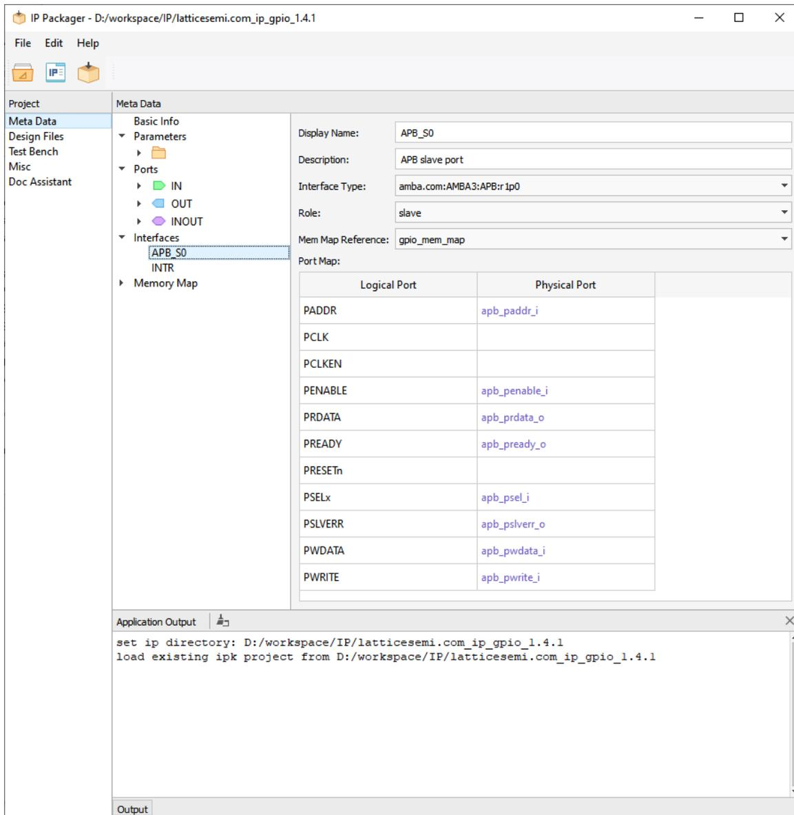
**Figure 3.22. Configure an Interface**
