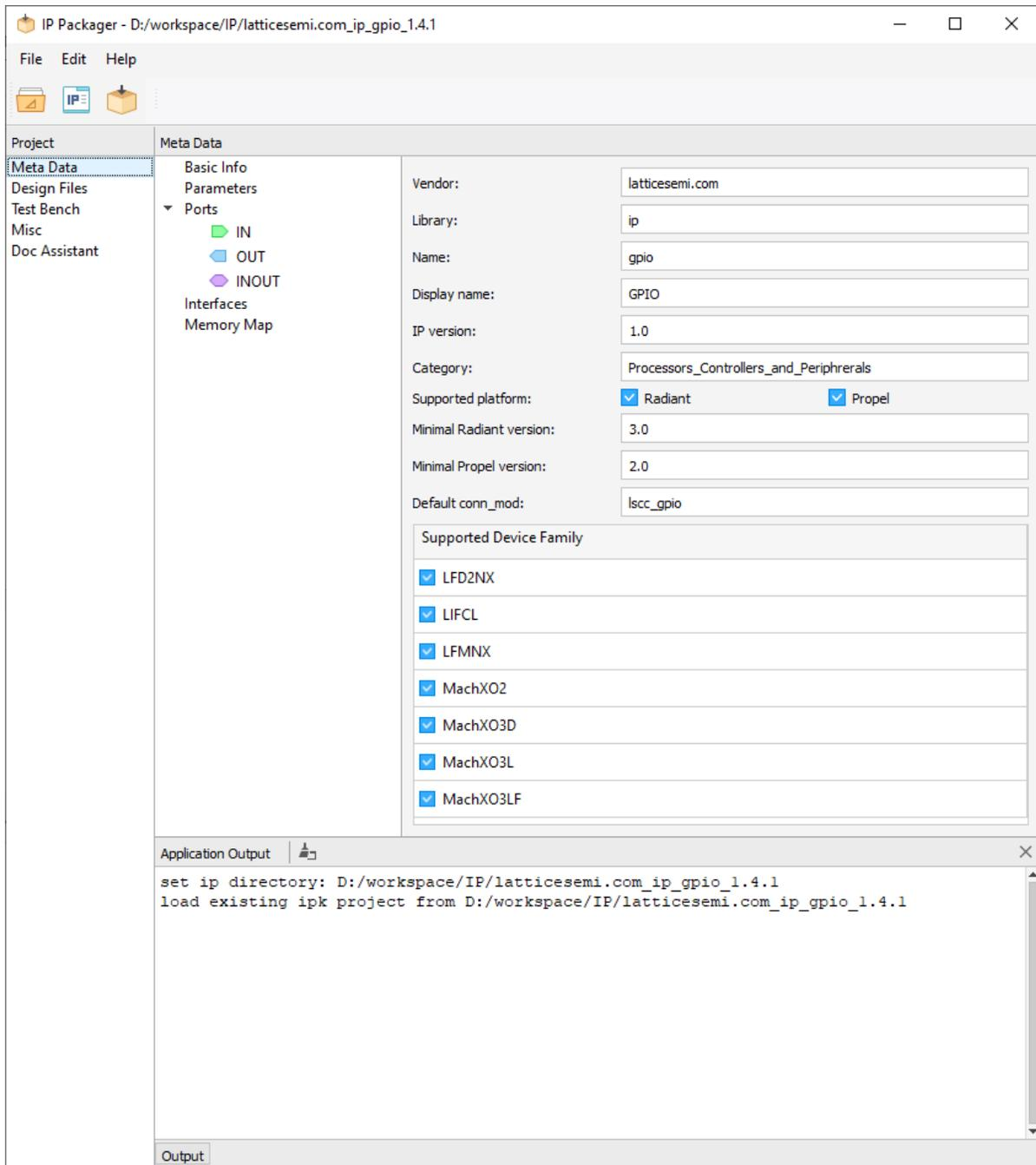
**Figure 3.5. IP Packager with IP Project Details**
