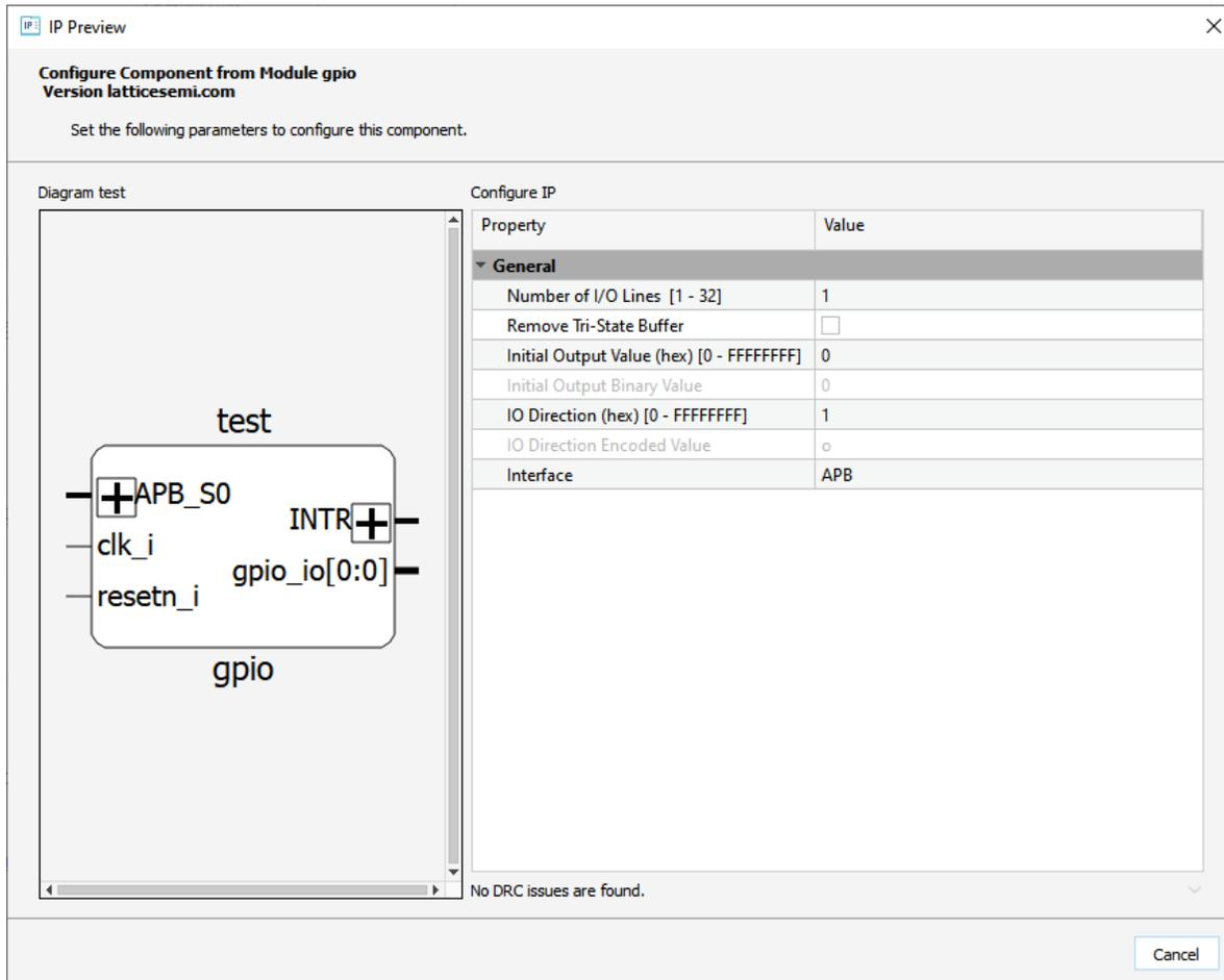
Figure 3.30. IP Preview Shows Configuration for IP Module
