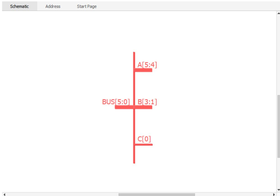
Figure 2.30. Schematic View Shows Split Module
