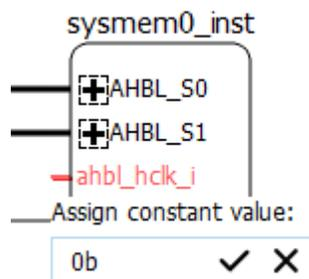
Figure 2.48. Dialog Box of Assigning Constant Value to an Input Pin
