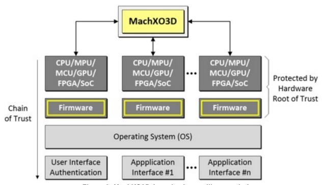
Figure 3. MachXO3D-based cyber resiliency solution.
