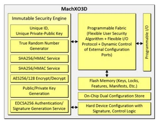
Figure 2. The MachXO3D secure control FPGA is the system's first-on, last-off, HRoT programmable logic device.
