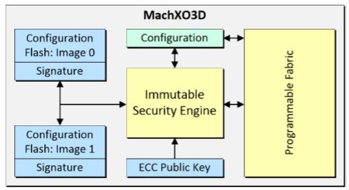
Figure 4. In addition to fully addressing the requirements of NIST SP 800 193 for cyber resiliency, the MachXO3D's dual-boot capability is key to securing the supply chain.
