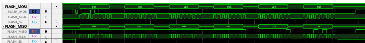
Figure 6.3. SPI Transaction Waveform During Device ID Command (S25L116K)
