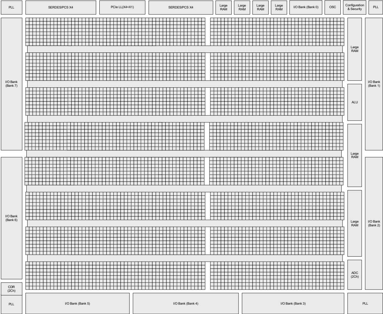
Figure 2.2. Simplified Block Diagram, LFCPNX-100 Device (Top Level)
