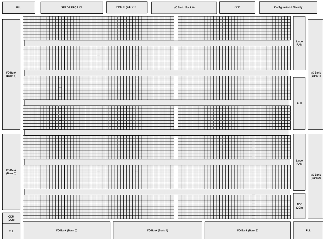
Figure 2.1. Simplified Block Diagram, LFCPNX-50 Device (Top Level)
