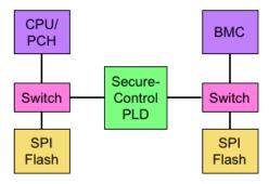
**Figure 1. PFR system architecture.** A secure-control PLD can implement PFR functions including SPI monitoring as well as handle control functions.
