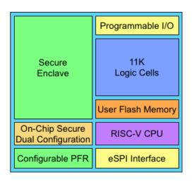
**Figure 2. Mach-NX block diagram.** The new chip includes a hard RISC-V CPU, a hard security block, Flash memory, programmable logic, and copious I/Os.
