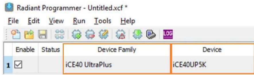
Figure 8.11. Lattice Radiant Programmer: Device Family and Device Setting
