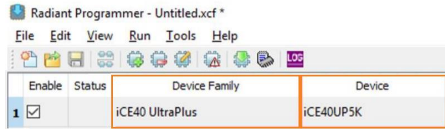
Figure 8.10. Lattice Radiant Programmer: Device Family and Device Setting
