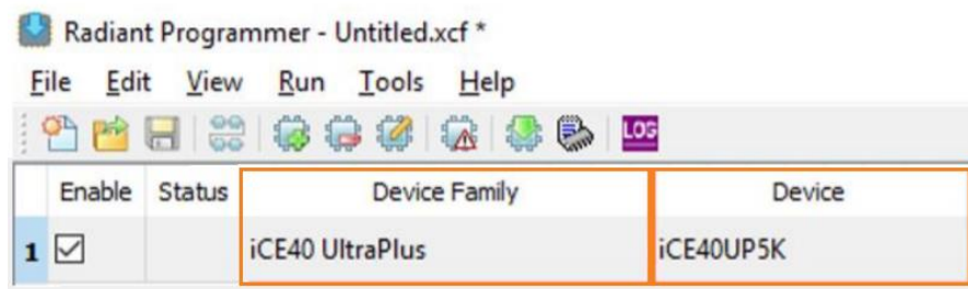
Figure 8.9. Lattice Radiant Programmer: Device Family and Device Setting
