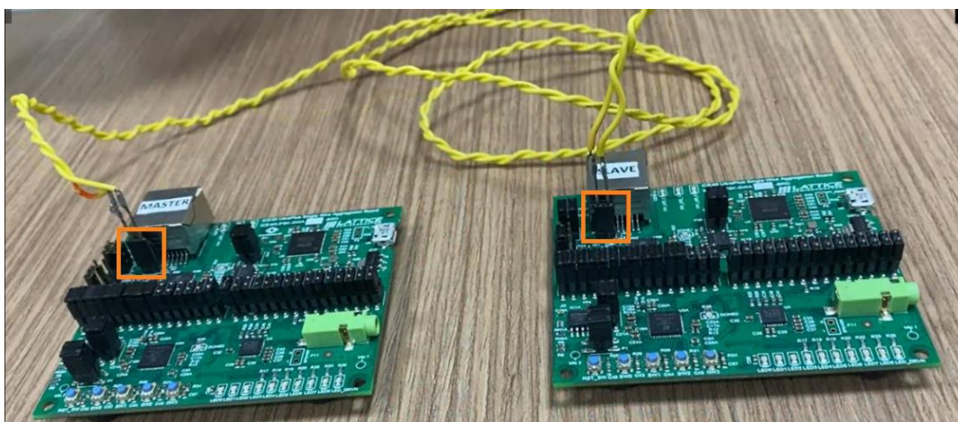
Figure 8.12. Connecting Single-Wire Link and Common Ground at Port P4
