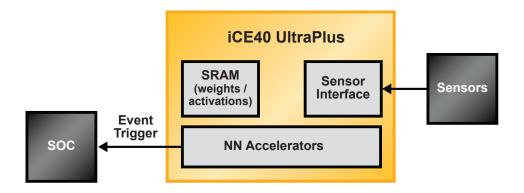
In this implementation, the sensor interface collects the inputs from the individual sensors, processing them in neural-network (NN) accelerators within the FPGA, assisted by on-chip SRAM that stores the weights and activations required for processing the neural nets. Decisions made by the accelerators can then wake the SoC if necessary for further processing.
