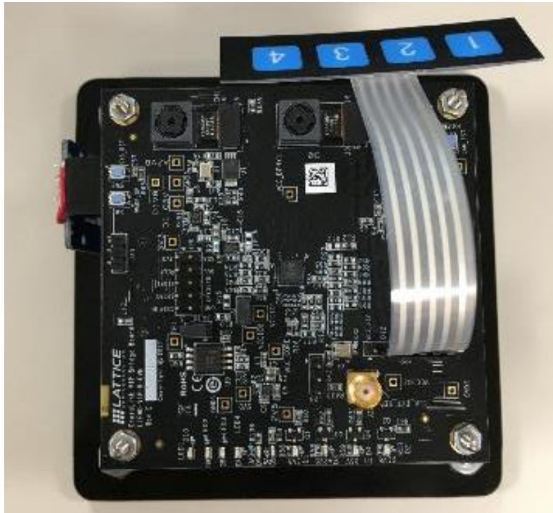
Figure 5.1 Attaching 1 × 4 Membrane Keypad to CrossLink VIP Bridge Board
