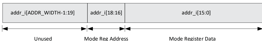
Figure 2.8. User-to-Memory Address Mapping for MR Programming
