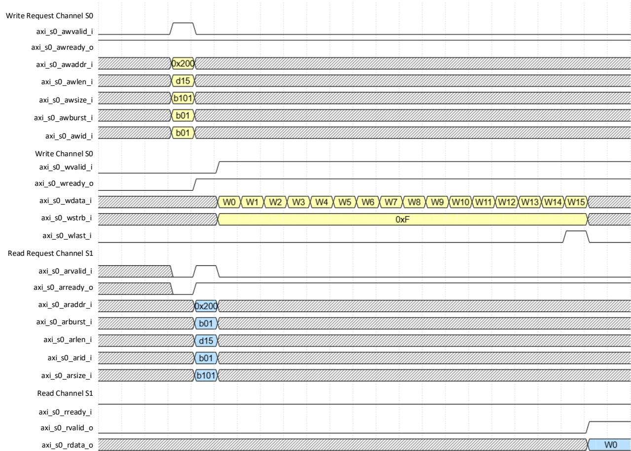
Figure 2.4. Dual Port AXI Interface (Read Arbitration)
