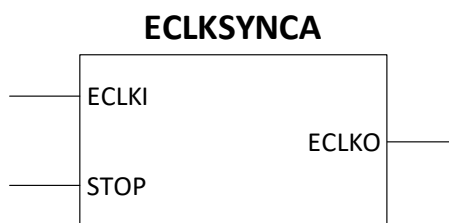
Figure 8.1. ECLKSYNCA Primitive Symbol
