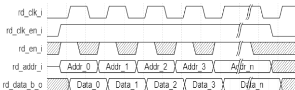
Figure 2.9. ROM Timing Diagram, without Output Registers
