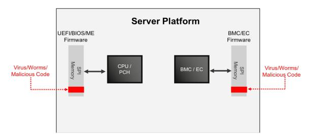
Figure 1: Unified Extensible Firmware Interface (UEFI) and the Baseboard Management Controller (BMC) interfaces offer limited firmware protection.
