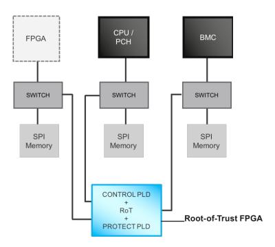
Figure 5: The RoT FPGA integrates the functions of the RoT MCU, Control PLD and the Protect PLD in a single-chip solution that is robust, scalable and impossible to bypass. In a server with a PFR-compliant PLD, the PLD's performance can monitor all component firmware in parallel without the need for additional FPGAs.
