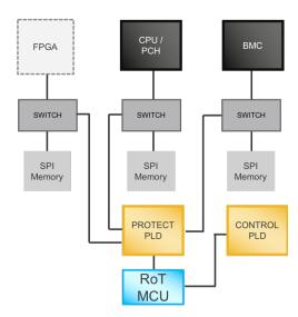
Figure 4: A PFR compliant server using an MCU for root of trust requires additional components (FPGAs) to provide performance if components are to boot simultaneously; a solution that is not scalable for high volume server applications.
