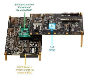
Figure 6: The Lattice FPGA RoT development toolkit features three boards: RoT FPGA development board, an ECP5 board to simulate a server's BMC and a SPI flash board to store the simulated BMC firmware.
