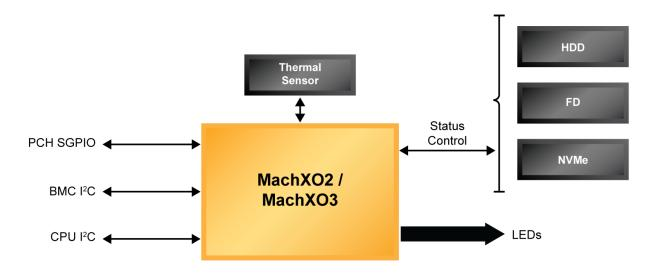
Fig. 4: Simplifying backplane control of hot swappable drives using MachXO2/MachXO3 PLDs
