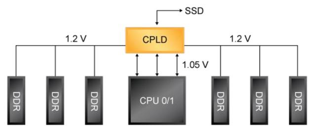
Fig. 9: MachXO2/O3 1V I/O supports the integration of I<sup>2</sup>C buffers
