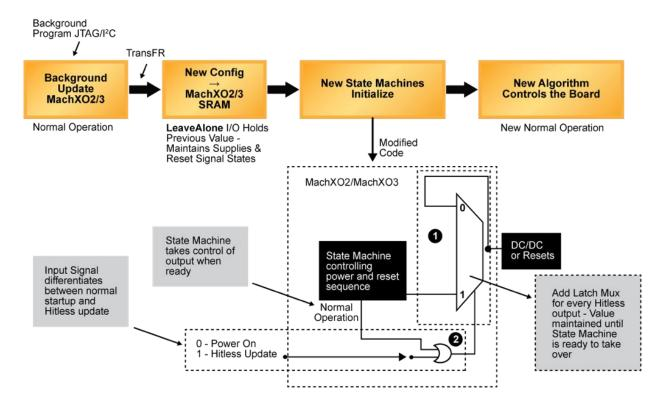
Fig. 3: How Hitless I/O works
