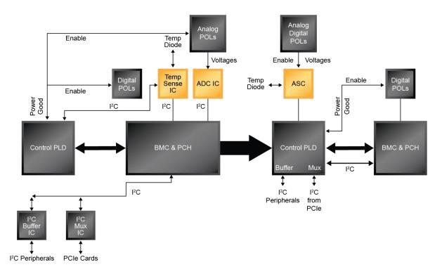
Fig. 6: New approach to integration of telemetry functions
