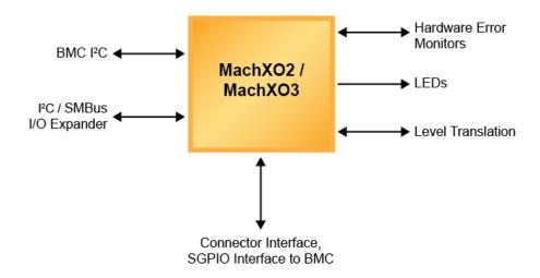
Fig. 5: Integration of host bus adapter logic
