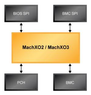
Fig. 7: MachX02/3-based solutions manages and validates BIOS and BMC firmware authentication
