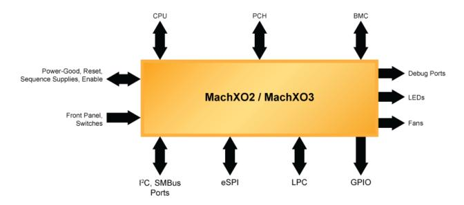
Fig. 2: Control PLDs based on the MachX02/MachX03
