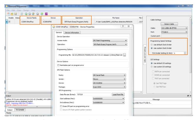
Figure 3.2. Programming Settings in Diamond Standalone Programmer
