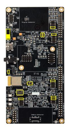
Figure 3.1. MDP Board with Configuration Locations Highlighted
