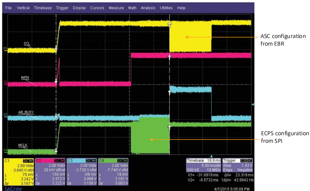
Figure 4.5. ECP5 Power-On-Reset with 62 MHz Quad-SPI and Compressed Bitstream
