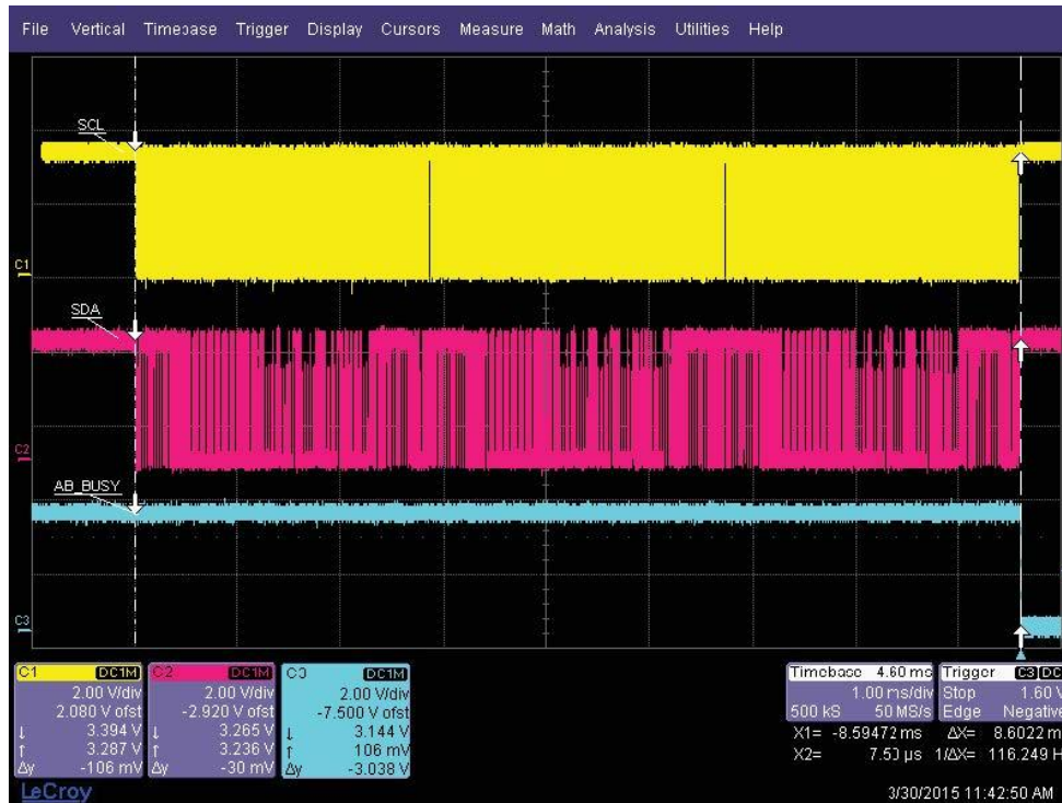
Figure 4.6. ASC Configuration Time for 3 ASCs using 400 kHz I 2 C Clock
