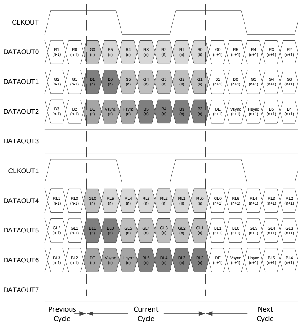
Figure 2.8. Dual Channel OpenLDI/FPD-LINK/LVDS Output Bus Waveform for RGB666 Format
