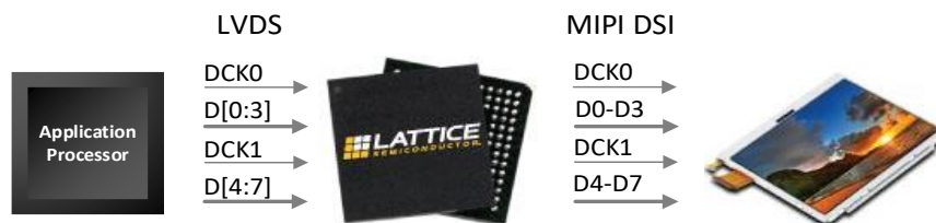
Figure 1.1. Sample OpenLDI/FPD-LINK/LVDS Receiver Interfaced to MIPI DSI System Diagram
