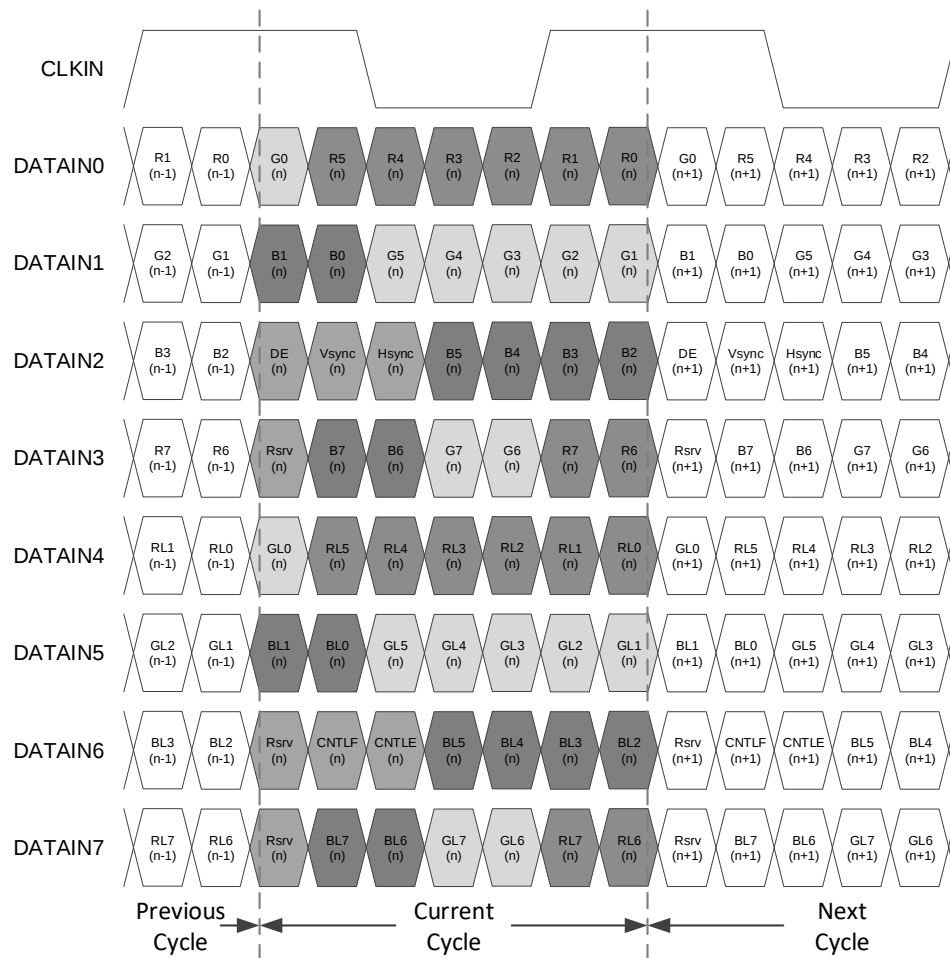
Figure 2.4. Dual Channel OpenLDI/FPD-LINK/LVDS Input Bus Waveform for RGB888 Format
