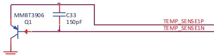
Figure 8.4. PNP Temperature Sensor Circuit
