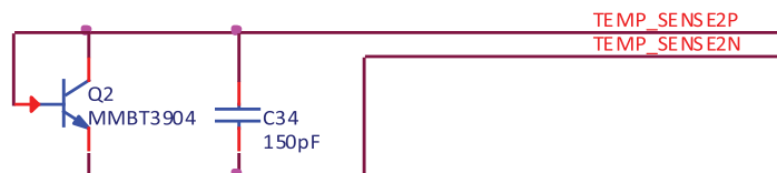
Figure 8.5. NPN Temperature Sensor Circuit
