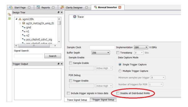
For a design that uses SED function, the "Disable all Distributed RAMs" box needs to be checked. If the existing Reveal module did not have Distributed RAM disabled, Reveal Inserter needs to be generated again to replace the existing Reveal module.
