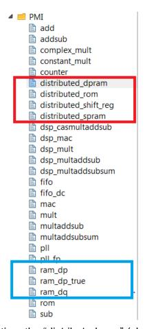
For a design that uses SED function, the "distributed\_xxx" (shown in red box) should <u>not</u> be used; EBR (shown in blue box) should be used instead. If the design is already using Distributed RAM, a new memory should be created with EBR to replace the existing one that is using Distributed RAM.
