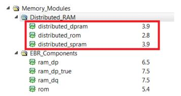
For a design that uses SED function, the "distributed\_xxx" (shown in red box) should <u>not</u> be used; EBR memory should be used instead. If the design is already using Distributed RAM, a new memory should be created with EBR to replace the existing one that is using Distributed RAM.
