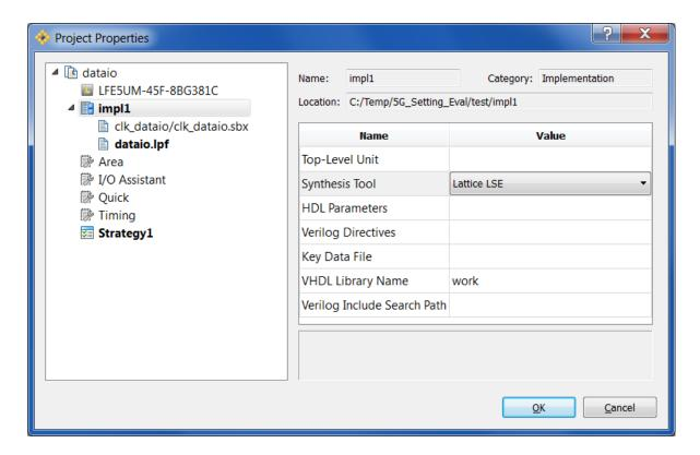
Set the "Synthesis Tool" setting to "Lattice LSE". Changing synthesis tool will require the modules generated in Clarity Designer to be re-configured. Once re-configured, customer can re-compile the design, and the Distributed RAM will be excluded.
