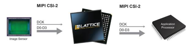
One Input to One Output MIPI CSI-2 Display Interface Bridge
