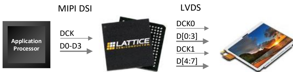
Figure 1.1. MIPI DSI to OpenLDI/FPD-Link/LVDS Interface Bridge System Diagram
