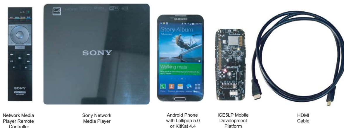
Figure 5. IR Self-Learning Demo Setup
