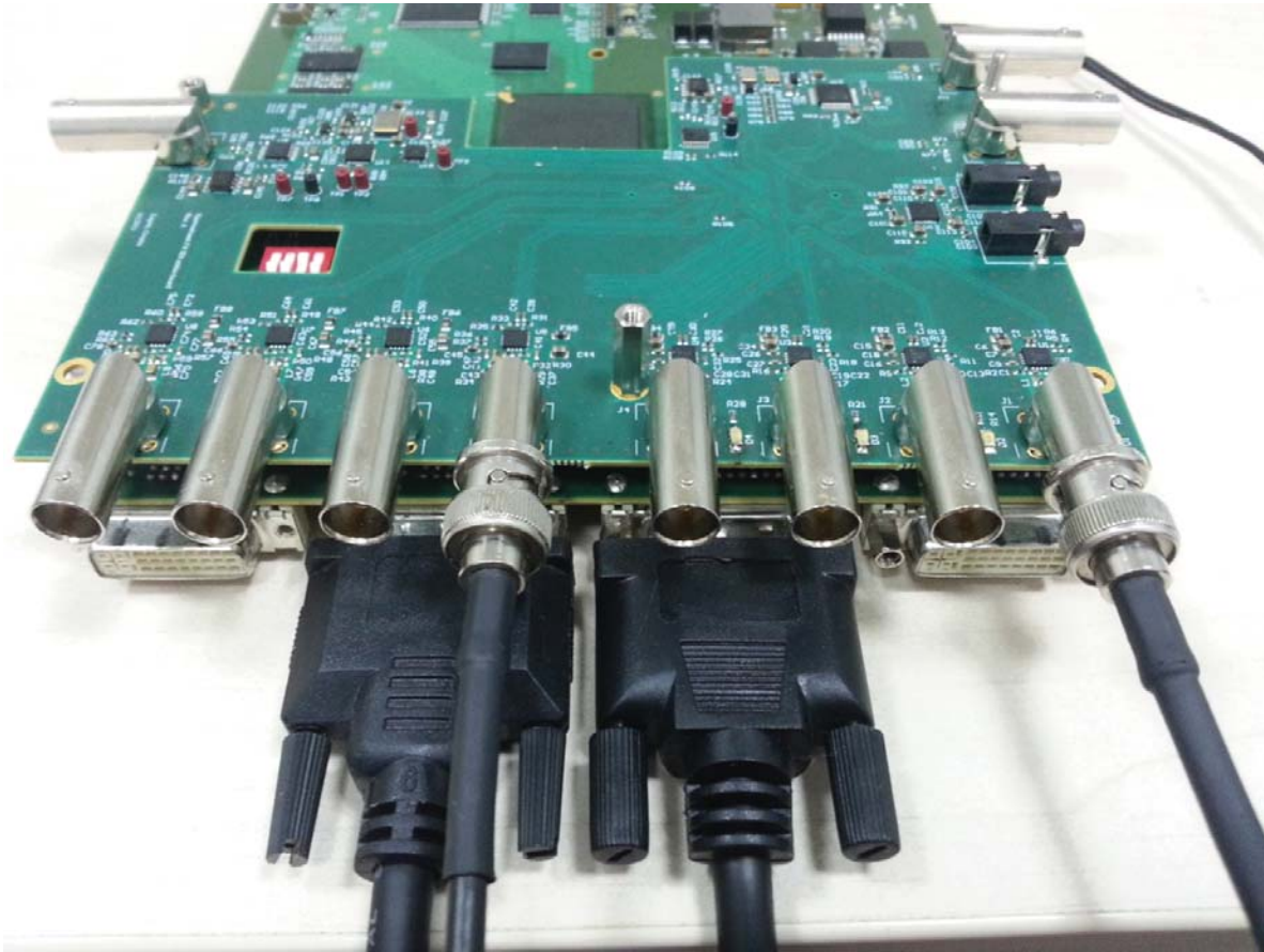
Figure 10. DVI Input, SDI Output to SDI Input Loopback, HDMI Output
