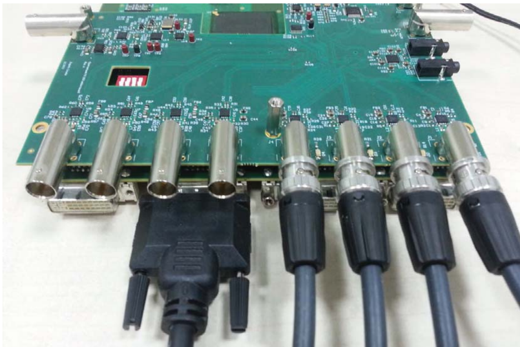
Figure 8. 4xSDI Input, DVI Output on Monitor with OSD
