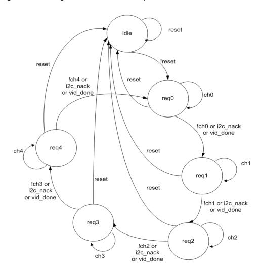
Figure 4: State Diagram of 5 VID channel Request
