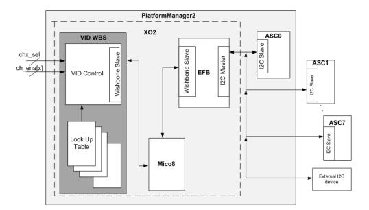
Figure 2: VID WISHBONE Slave Mode Block Diagram
